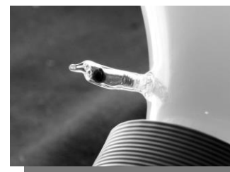
A small solid mercury amalgam ball is easily and safely snapped off for recycling. Magnets are recyclable metal and the remainder of the bulb is disposable glass.
