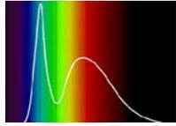
a high blue and UV bias that can be dangerous for humans and many animals. The LED spectrum is generally concentrated in the lower region with *insufficient light* within the most visually acute areas for human vision. Even filtered LEDs are usually deficient in the transition into green and yellow which are the most reactive wavelengths for the human eye. The effect is called
