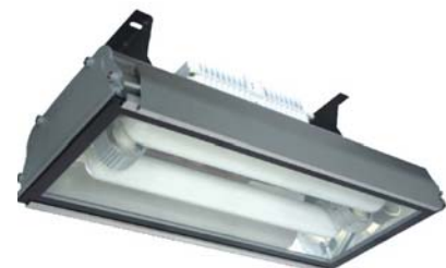
A 400-watt Snow-Bright “race-slope” lamp produces an elongated lighting pattern that can disperse light along the vertical slope contour. Unlike conventional spot lights, the light source is over 2 feet long. Lamps can be canted to accommodate specific slope incline.
